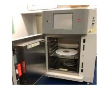
The self-contained, benchtop CellRad+ allows for *in vitro* radiation and programmable display for repeat irradiation protocols.
